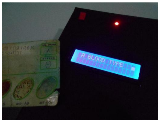
Fig 4. The accuracy is evaluated by matching the result with a blood type card released by IRC.
