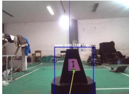
Fig. 10. Robot Object Detection with YOLOv5
